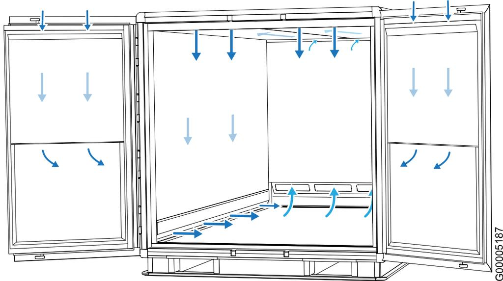
Fig. 4 Schematic view of the internal airflow
