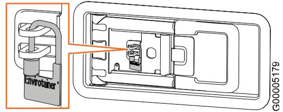
Fig. 23 Close, lock and seal the doors
