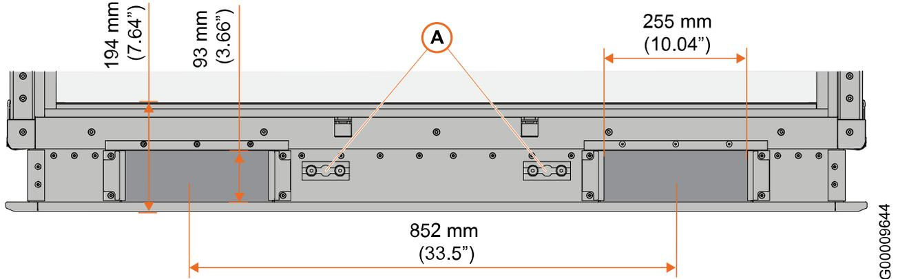
Fig. 9 Fork lift pockets and tie-down brackets
