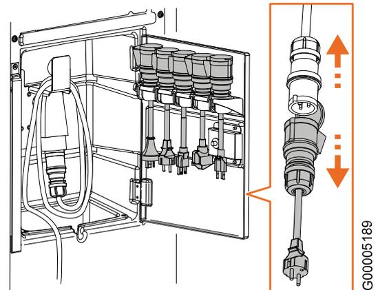
Fig. 31 Disconnect the adapter
