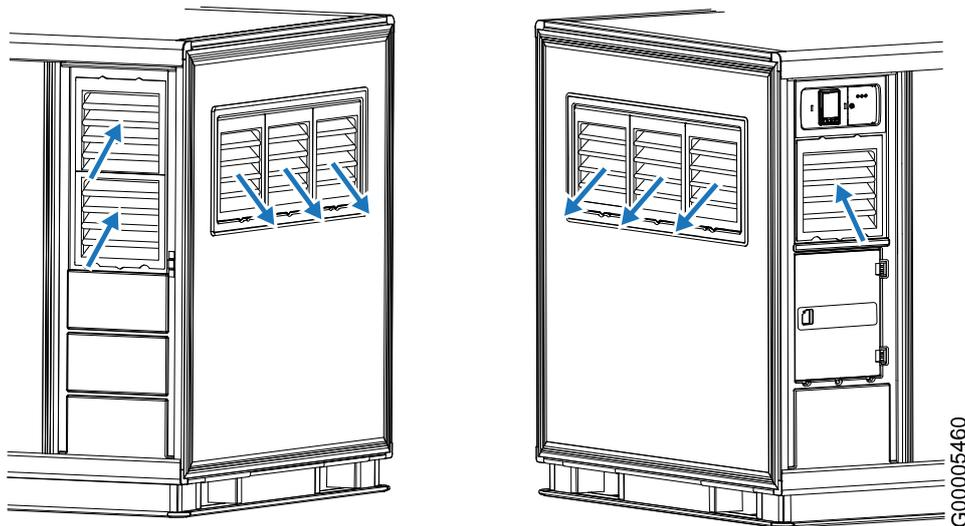
Fig. 5 Schematic view of the internal-external airflow transition (example: RelEye<sup>®</sup> RLP container)
