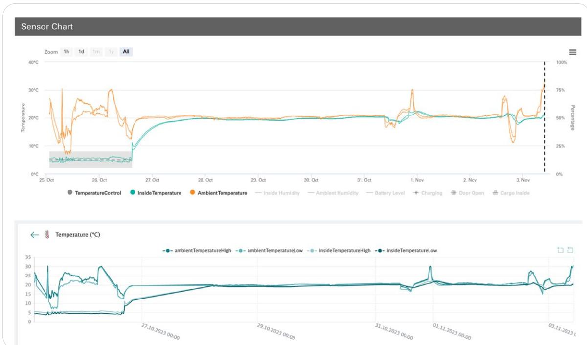
Comparison of temperature data from a live shipment in the Envirotainer Portal (top) and DB Schenker’s IoT system (bottom)
